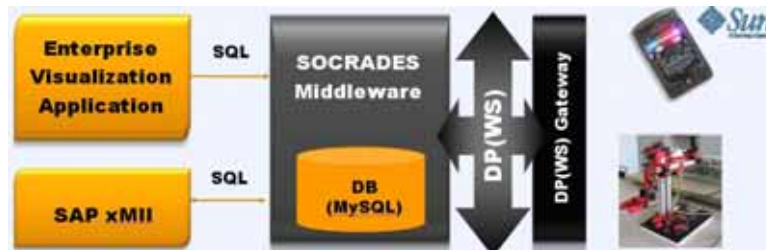
Figure 2 – Integration of Enterprise, Middleware and Device layers
