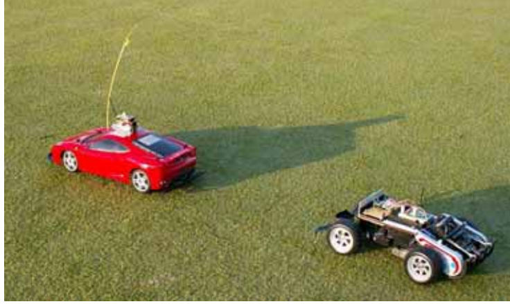
Fig. 2. The leader (left) and the follower (right) cars, equipped with sensor nodes and 3-D accelerometers and magnetic compasses.
