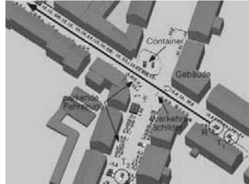
Figure 5. Three-dimensional model of the measuring scenario for the ascertainment of the Rice factor K [07]
